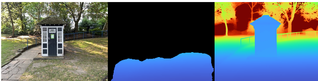
Fig. 1. Comparing inputs and output for monocular depth enhancement: The figure shows the source image (left), the sensor’s original depth map (center), and the improved metric monocular depth map after enhancement (right). In the depth maps, red colors signify points farther from the viewer. The depth maps use a colormap where red represents farther points.
